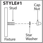
**STYLE#1**- Tuck electrical wires into outlet box and position fixture over studs on mounting bracket assembly. Secure fixture in place with star washers and cap nuts. **Note:** If required, assemble body and spread the arms of the fixture out evenly.
