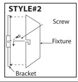
**STYLE #2** - Insert one screw into the mounting bracket - do not tighten yet. Tuck electrical wires into outlet box and position fixture over the mounting bracket. Line up the screw in the bracket to the "7" hole on the fixture. Slide fixture to secure in place. Insert remaining screw. Tighten both screws to secure.
